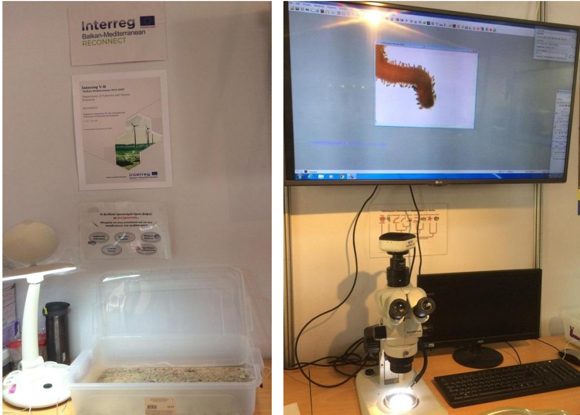
**Figure 6.** Mini benthic macrofauna laboratory (sorting and identification) (Photos MER Lab Ltd.).
